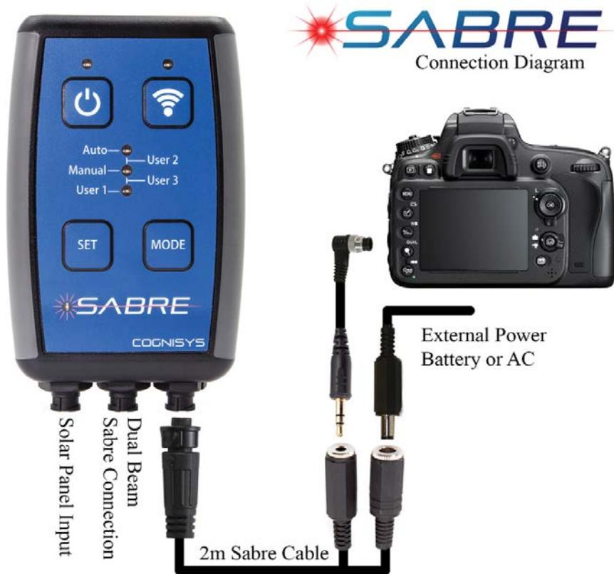
Figure 2 - Connection Diagram
