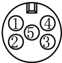
1. DC Power In (See specifications for the voltage range in section 11)
