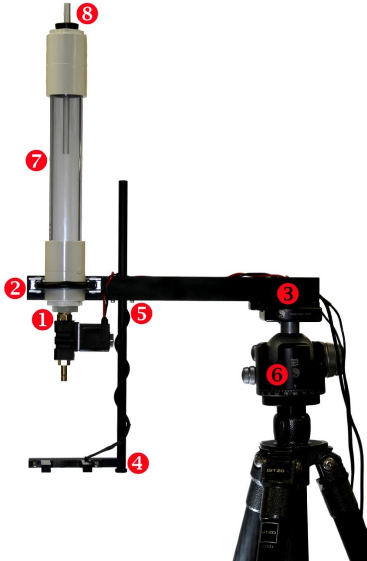
1. Thread the Mariotte Siphon to the water valve from the Water Valve Assembly
