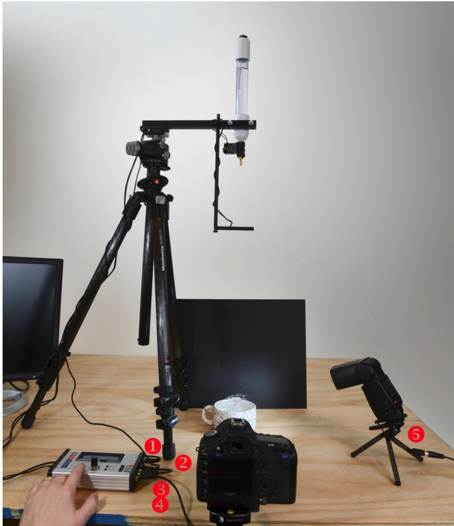
1. Connect the supplied AC adapter to your mains and connect the 2.1mm power connector to StopShot. StopShot will go through the power up sequence as soon as power is applied.
