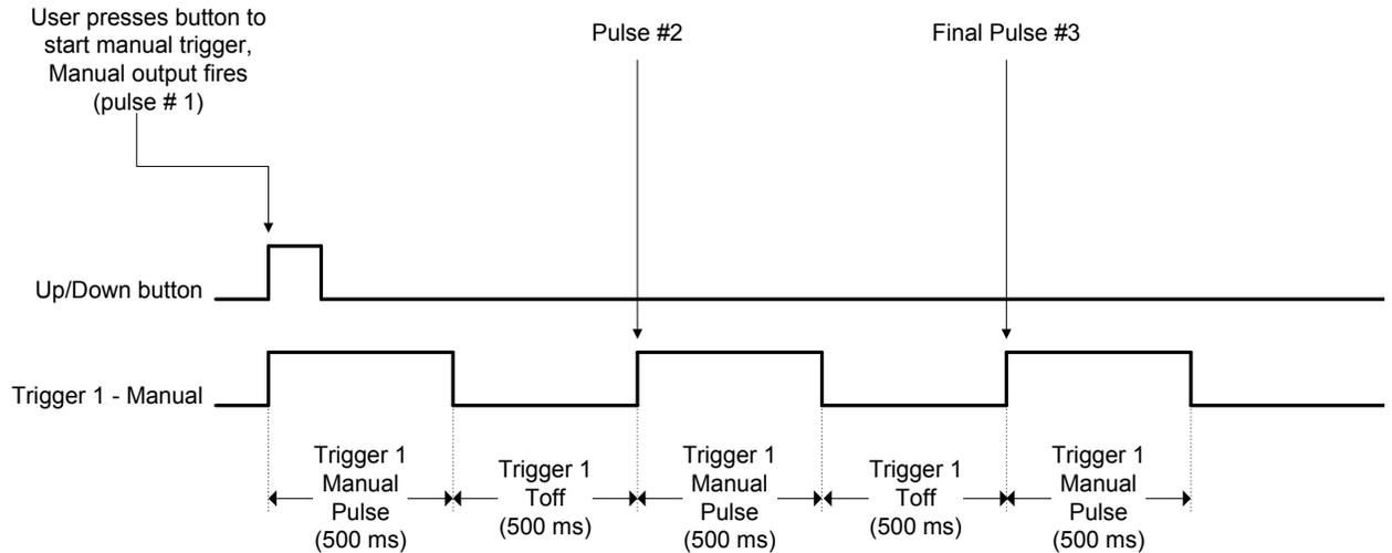
Figure 7 - Manual Mode Timing Diagram
