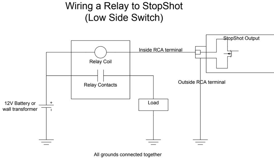
Figure 16 - Wiring an external relay
