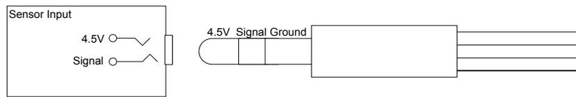
Figure 14 - Sensor Connection
