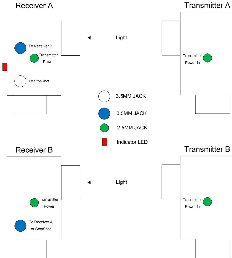
Figure 17 - Cross-beam connections
