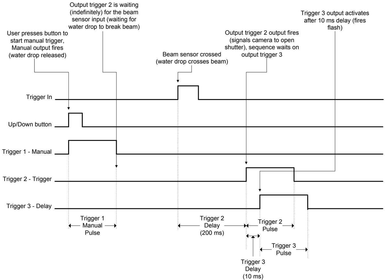
Figure 10 - Sequential Mode Timing Diagram
