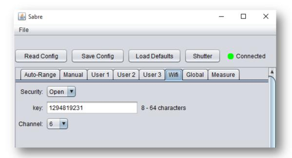
After making changes here be sure to press the "Save Config" button at top to permanently save the settings. They will not take effect until either Wifi or power is turned off and then back on. This is to prevent loss of communication immediately upon changing these values.
