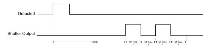
Figure 3 - Shutter Timing Diagram
