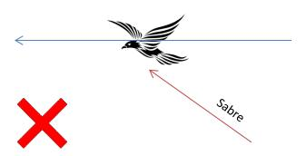
Avoid shooting through glass. If that is unavoidable, make sure that Sabre is pushed directly to the glass. Otherwise the distance measured can drift between the glass and what is outside the glass, causing false triggers.
